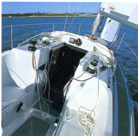
In keeping with Dehler's modern tradition, just two winches control the boat in standard form
